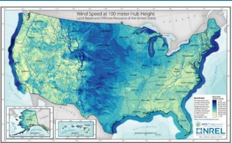
U.S. Land-Based and Offshore Wind Resources Annual Average Wind Speed at 100 Meters Above the Ground
