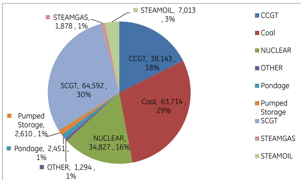
Figure 3-3: Starting 2% BAU Scenario Capacity Mix without Wind and Solar (MW)
