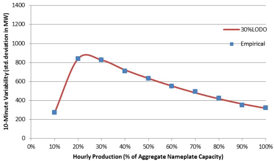
Figure 1-75: Statistical Characterization of 10-Minute PV Variability for The 30% LODO Scenario
