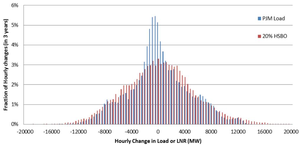
Figure 1-42: Hourly Change in PJM Load and Net Load For 20% HSBO Scenario (3 Years of Data)
