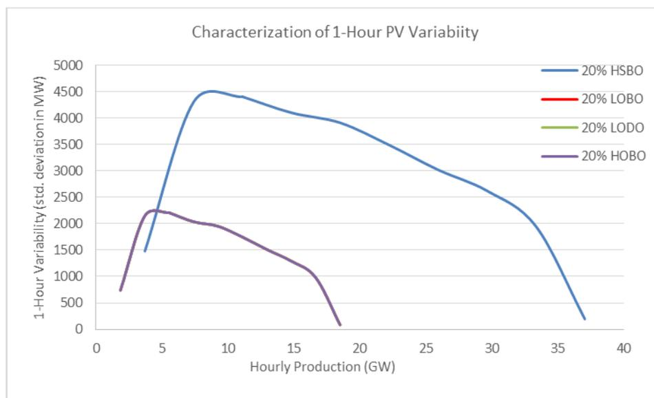
Figure 1-88: Expected 1-Hour Persistence Forecast Error as Function of Current PV Production Level For 20% Scenarios (Note LOBO, LODO and HOBO Scenarios Use Same PV Sites)
