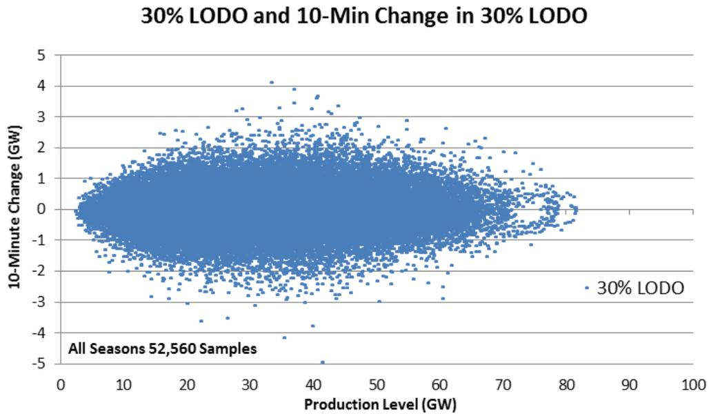
Figure 1-54: 10-Minute Wind + Solar Variability as a Function of Production Level For 30% LODO Scenario
