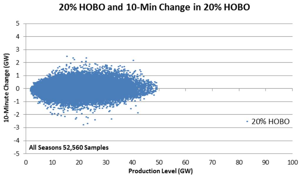
Figure 1-49: 10-Minute Wind + Solar Variability as a Function of Production Level For 20% HOBO Scenario
