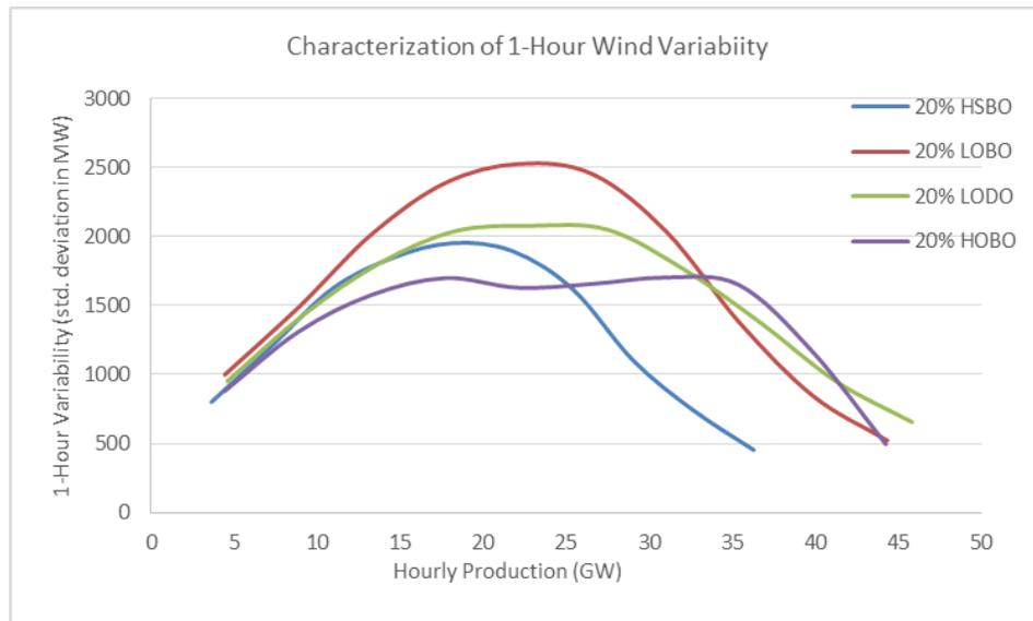
Figure 1-87: Expected 1-Hour Persistence Forecast Error as Function of Current Wind Production Level For 20% Scenarios
