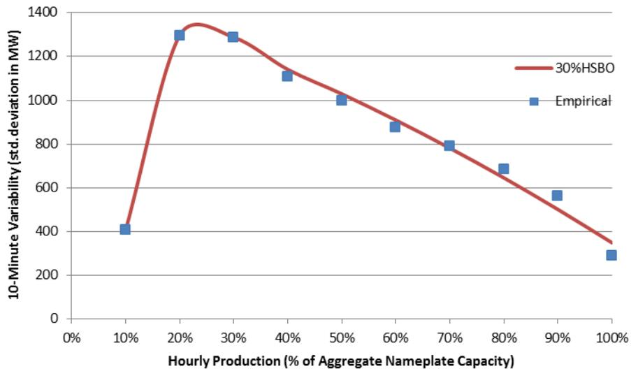
Figure 1-73: Statistical Characterization of 10-Minute PV Variability for The 30% HSBO Scenario
