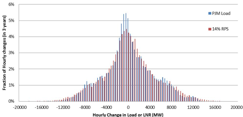
**Figure 1-40: Hourly Change in PJM Load and Net Load For 14% RPS Scenario (3 Years of Data)**
