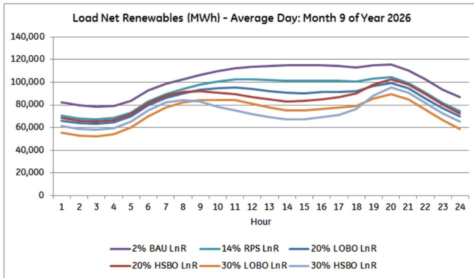
Figure 3-18: Load Net Renewables for a Day in September 2026 with the Largest HSBO LnR Range
