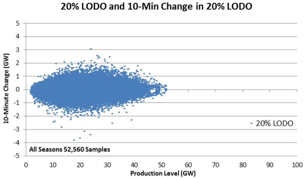
Figure 1-50: 10-Minute Wind + Solar Variability as a Function of Production Level For 20% LODO Scenario
