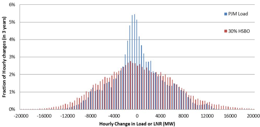
Figure 1-44: Hourly Change in PJM Load and Net Load For 30% HSBO Scenario (3 Years of Data)
