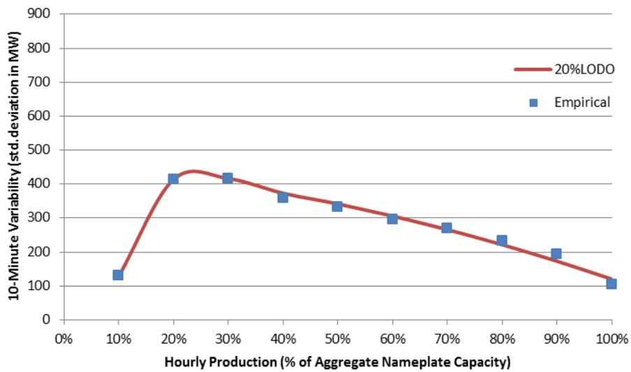
Figure 1-71: Statistical Characterization of 10-Minute PV Variability for The 20% LODO Scenario
