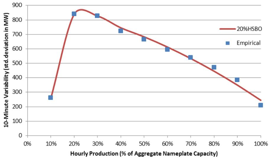
Figure 1-69: Statistical Characterization of 10-Minute PV Variability for The 20% HSBO Scenario
