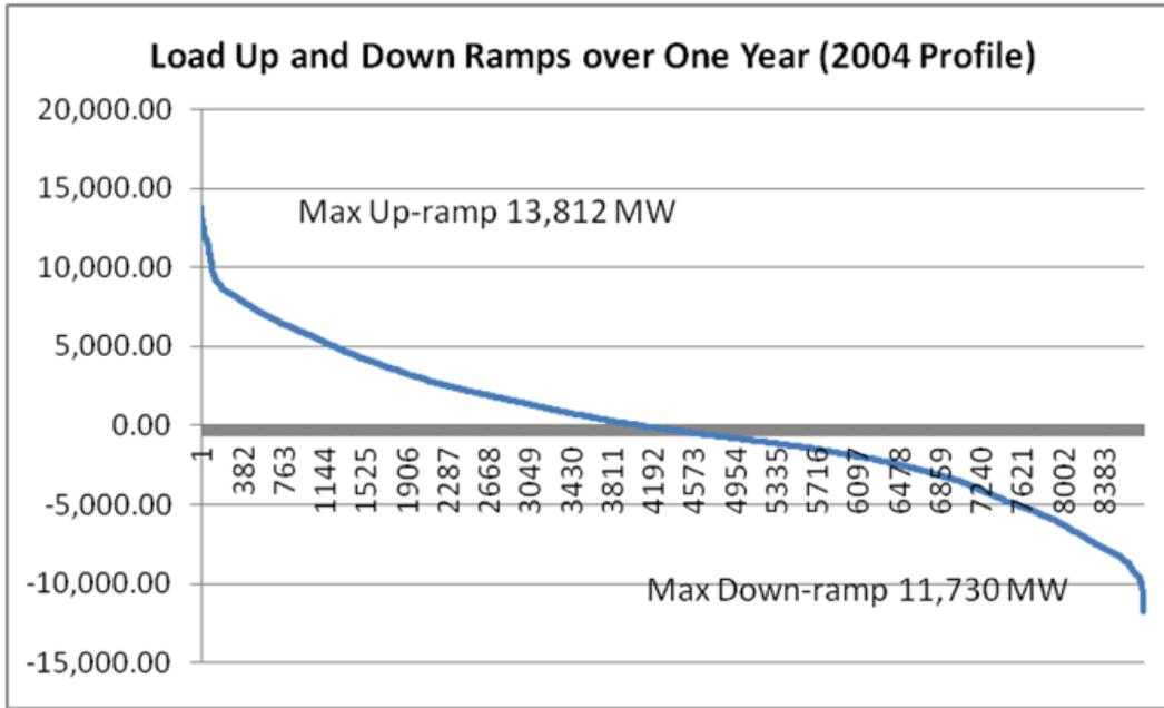
Figure 1-8: Hour To Hour Load Ramp Duration Curve for Study Year with 2004 Profile
