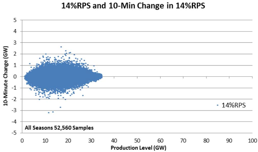
Figure 1-48: 10-Minute Wind + Solar Variability as a Function of Production Level For 14% RPS Scenario
