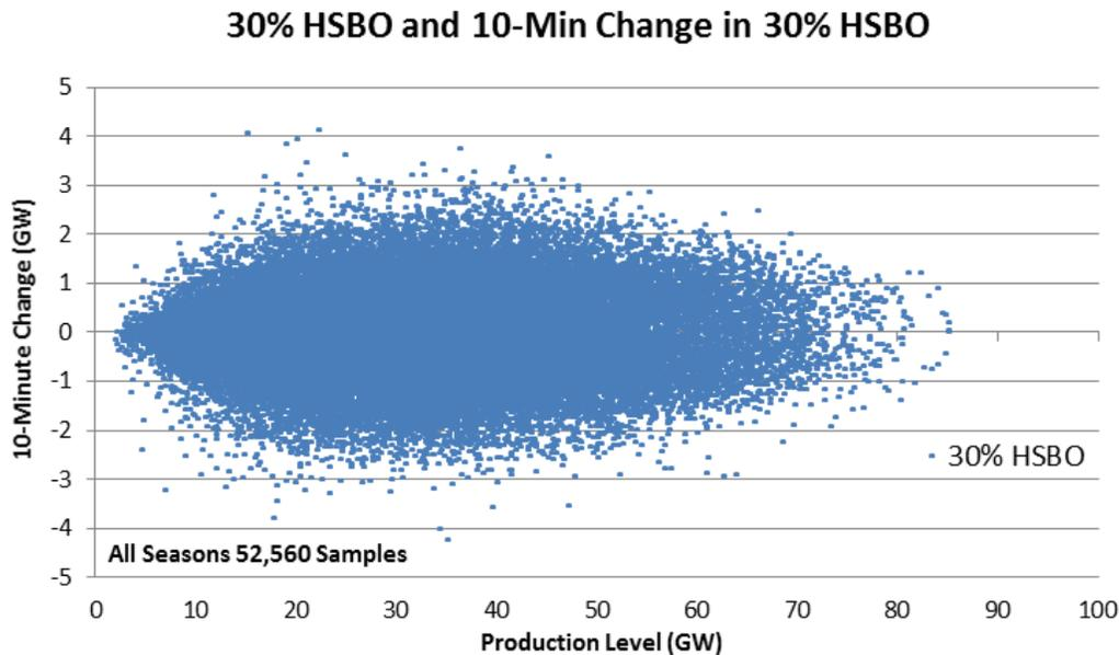
**Figure 1-56: 10-Minute Wind + Solar Variability as a Function of Production Level For 30% HSBO Scenario**
