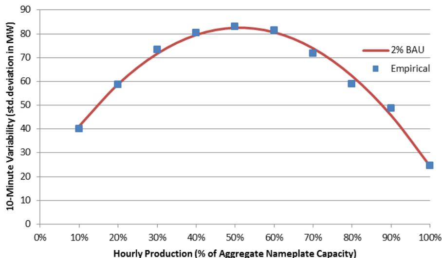
Figure 1-57: Statistical Characterization of 10-Minute Wind Variability for The 2% BAU Scenario
