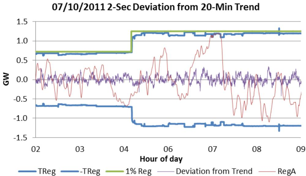
Figure 2-2: Metered Regulation for July 10, 2011 with 2 Second Deviations from a 20-Minute Trend
