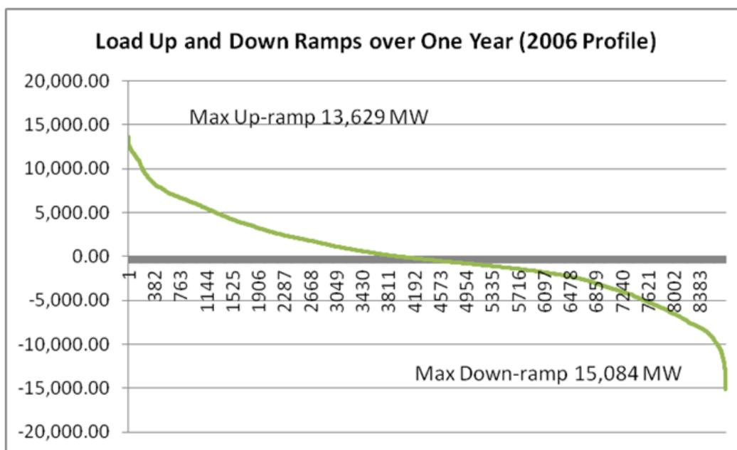
Figure 1-10: Hour To Hour Load Ramp Duration Curve for Study Year with 2006 Profile
