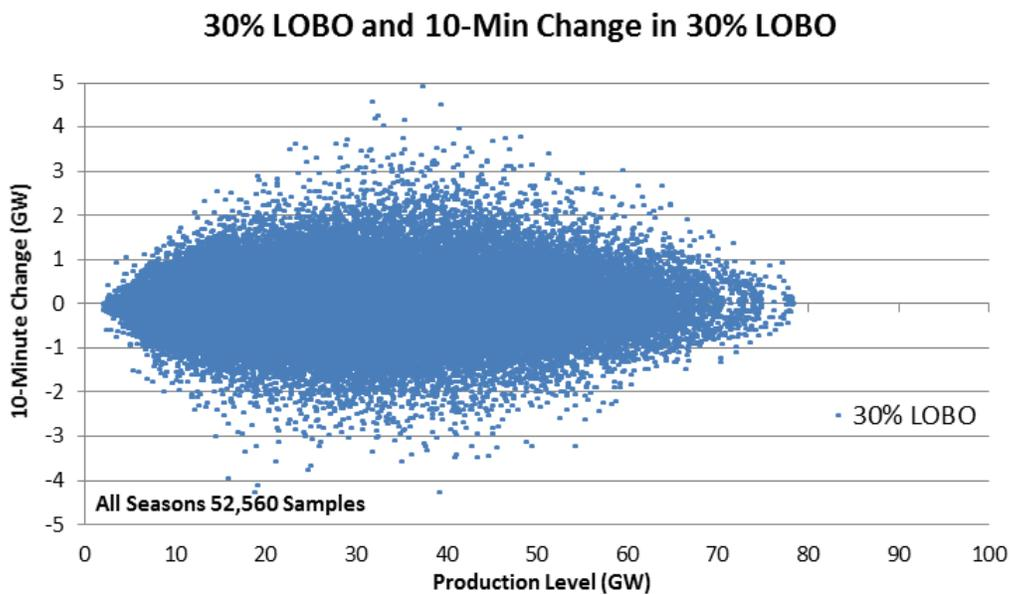
Figure 1-55: 10-Minute Wind + Solar Variability as a Function of Production Level For 30% LOBO Scenario
