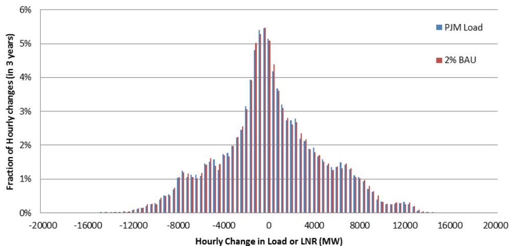
**Figure 1-39: Hourly Change in PJM Load and Net Load For 2% BAU Scenario (3 Years of Data)**
