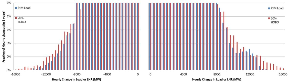
**Figure 1-45: Distribution Tails of Hourly Changes for PJM Load and Net Load for 20% HOBO Scenario**
