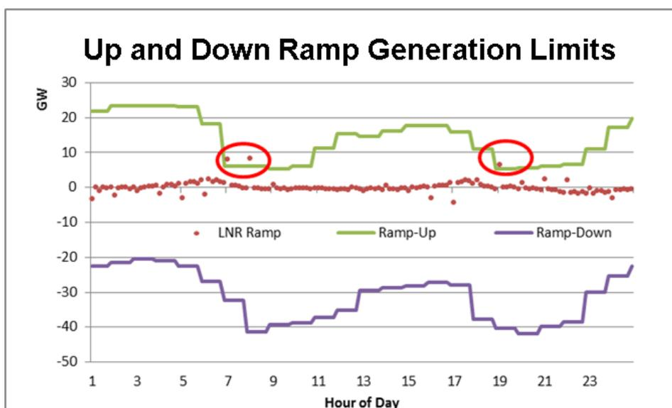
Figure 2-10: Sample Day Showing 10-Minute Periods That Exceed Ramp-Up or Ramp-Down Limits
