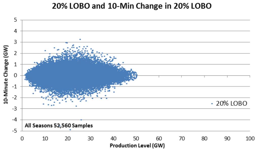
Figure 1-51: 10-Minute Wind + Solar Variability as a Function of Production Level For 20% LOBO Scenario
