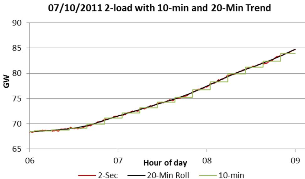
Figure 2-3: 2-Second Load Data Plotted with 20-Minute Rolling Average and 10-Minute Average Load
