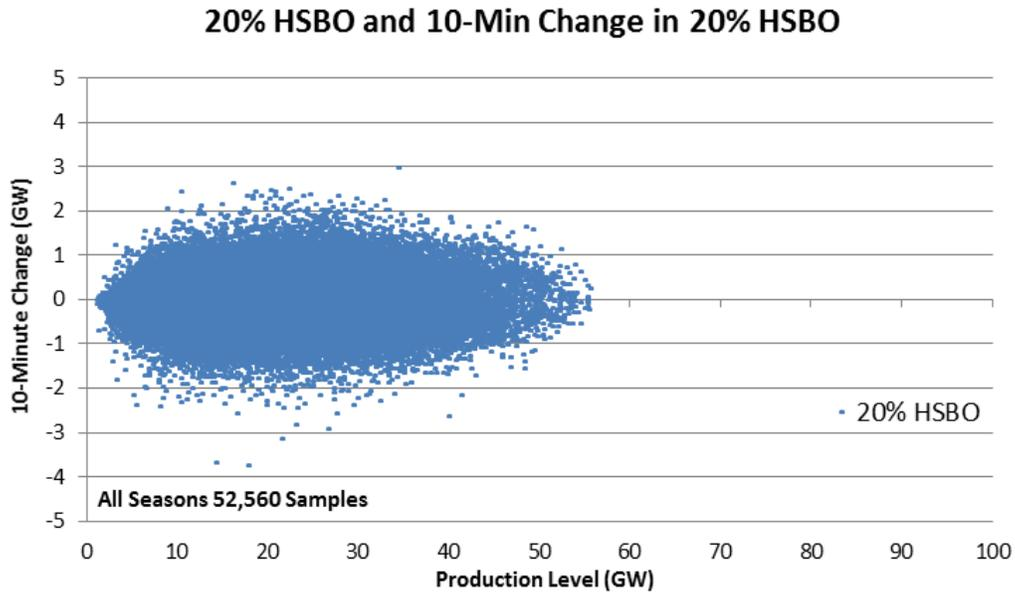
Figure 1-52: 10-Minute Wind + Solar Variability as a Function of Production Level For 20% HSBO Scenario
