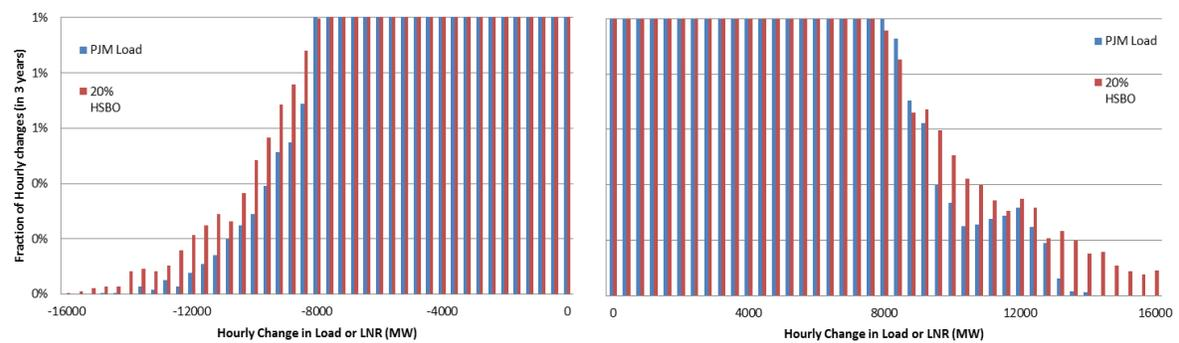
**Figure 1-46: Distribution Tails of Hourly Changes for PJM Load and Net Load for 20% HSBO Scenario**
