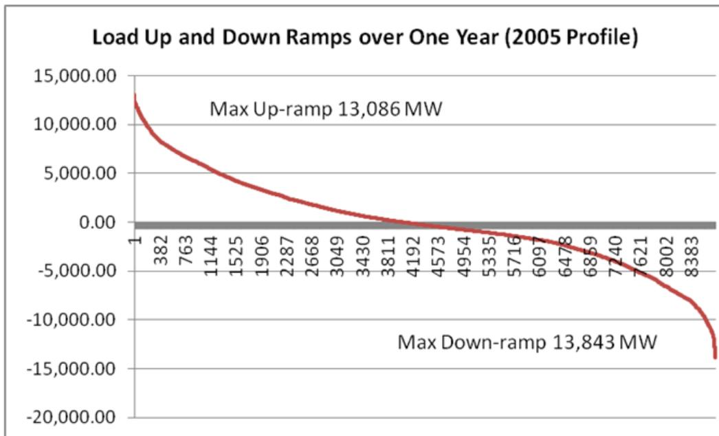
Figure 1-9: Hour To Hour Load Ramp Duration Curve for Study Year with 2005 Profile
