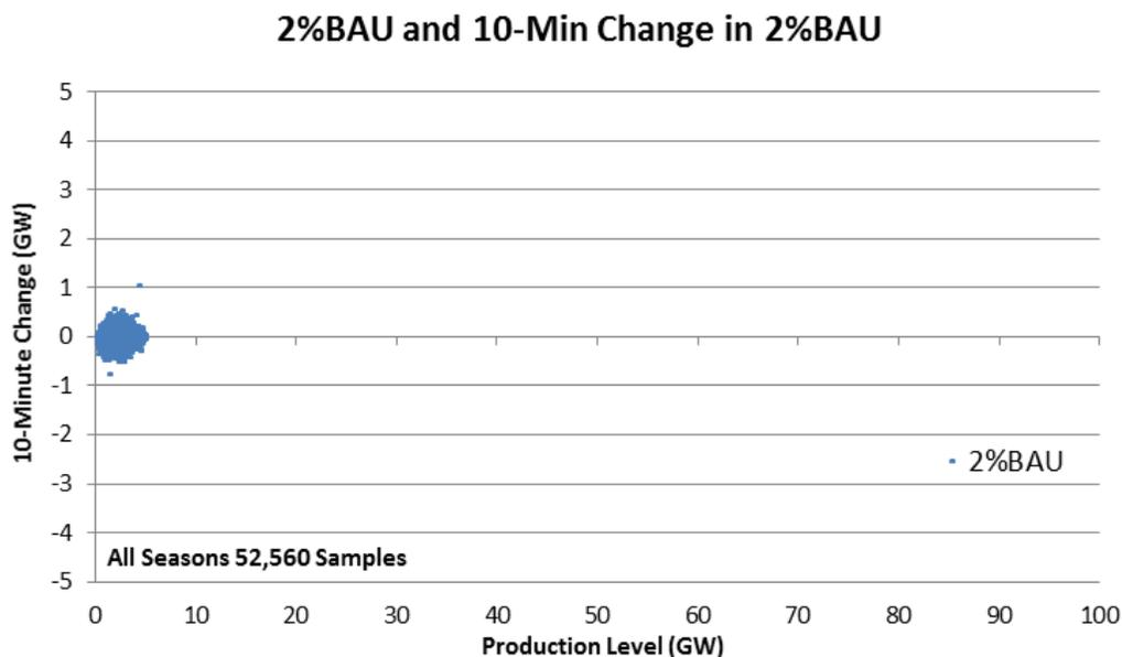
**Figure 1-47: 10-Minute Wind + Solar Variability as a Function of Production Level For 2% BAU Scenario**
