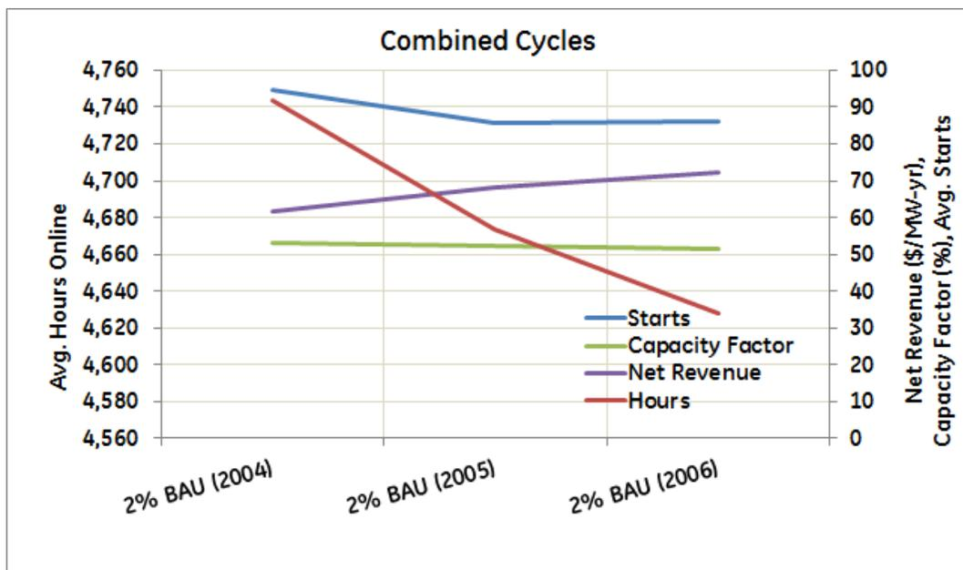
Figure 2-17: Variation in Performance of CCGT units under Different Profile Years (2% BAU Scenario)
