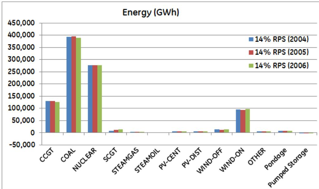
Figure 2-2: Variation in Generation by Unit Type under Different Profile Years (14% RPS Scenario)
