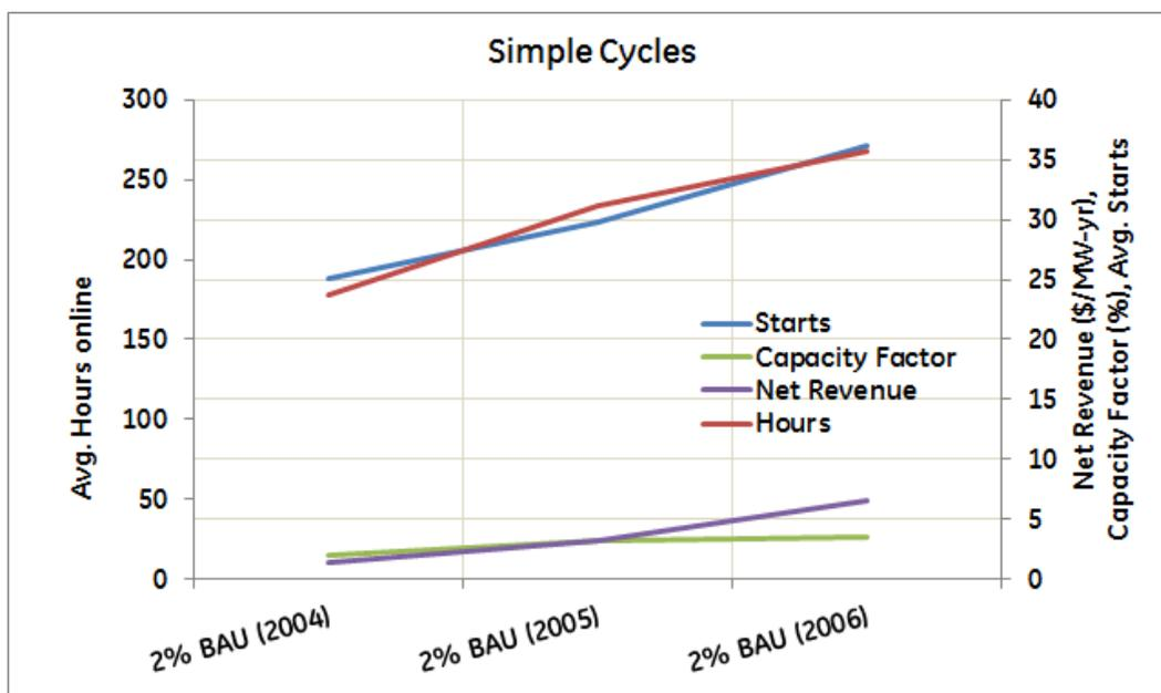
Figure 2-19: Variation in Performance of SCGT units under Different Profile Years (2% BAU Scenario)
