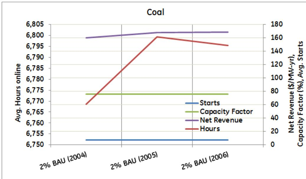
Figure 2-18: Variation in Performance of Coal units under Different Profile Years (2% BAU Scenario)
