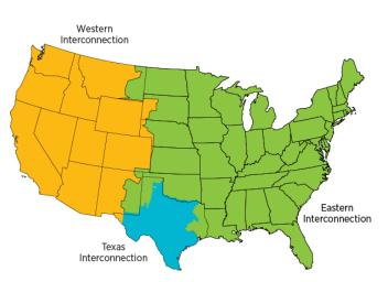
is no other part of the interconnection that is available to connect in order to synchronize the isolated part of the grid to the rest of the operating grid. In such an instance, we call on black start resources, which are generators
